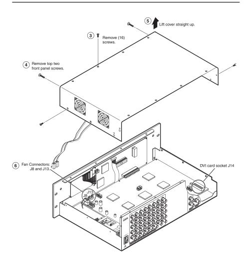
Figure 1 — Removing the switcher cover
